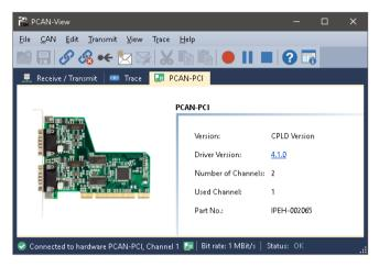
Figure 13: PCAN-PCI tab (example)
