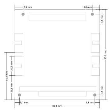
Figure 16: Dimension drawing PCAN-PC/104-Plus Quad.
