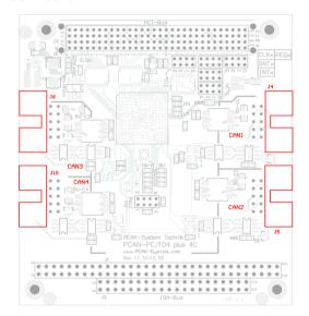
Figure 2: Position of the sockets for the CAN connection, J4 for CAN channel 1 (upper right position), J5 for CAN channel 2 (lower right position), J6 for CAN channel 3 (upper left position), J10 for CAN channel 4 (lower left position)
