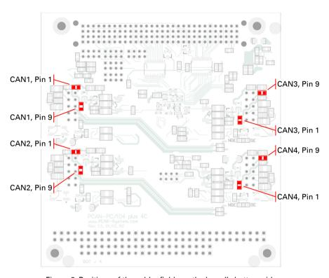
Figure 6: Positions of the solder fields on the board's bottom side for a 5-Volt supply at the CAN connection (D-Sub)
