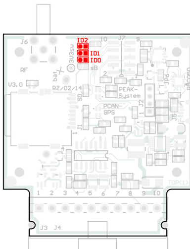
Solder fields for coding solder jumpers on the circuit board
